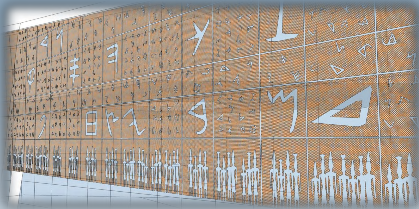
A Perforated Metallic Sheet Skin Along the Western/Southern Elevations
